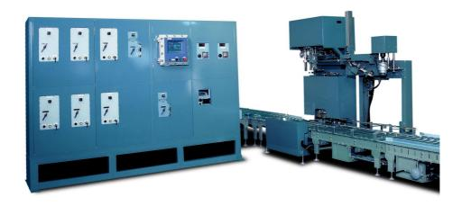
\*Over capper-with conveyor line at front and back
